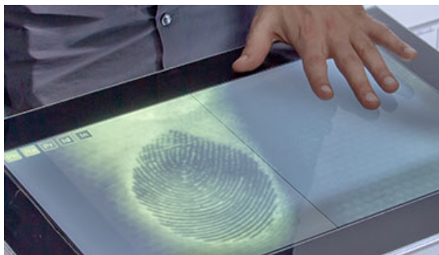
Figure 3: Fiberio displaying a region of its high-resolution raw input image, revealing the user’s fingerprint.
