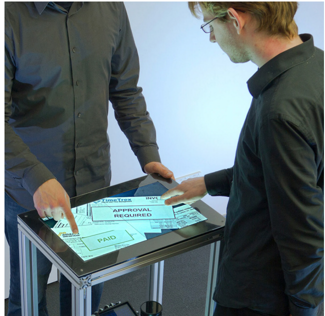
Figure 1: Fiberio is a rear-projected tabletop system that identifies users based on their fingerprints during each interaction —unobtrusively and securely. The shown application uses this to verify that the respective user has the authority to perform the current activity, here approve invoices above a certain value. The key that allows Fiberio to display an image and sense fingerprints at the same time is its screen material: a fiber optic plate.
